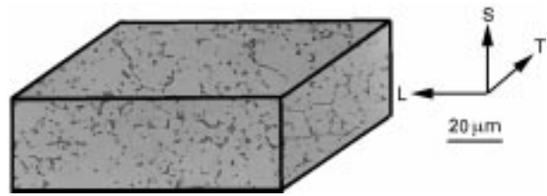
Figure 9 Microstructure of Ti alloy in IMI 834 materials. IMI 834-SM1140 + MMC is shown, but all the others are similar.
